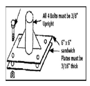
NOTE (Option #1): The bolts used to sandwich the cage to the floorpan must be a minimum of grade 8 material.
