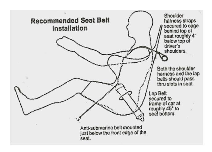
All brackets must be installed in direction of pull to avoid excessive stress to the anchor points during driving [fatigue stress] or during an accident.
