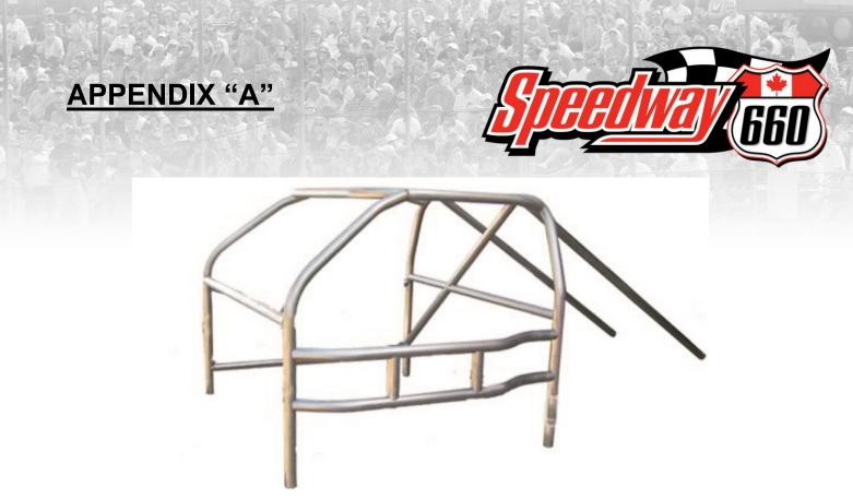
**NOTE**: Optional - Right side pipes may be in the form of an "X" or a single tube angled down from top of door on the right rear pipe to the bottom of the right front pipe.
