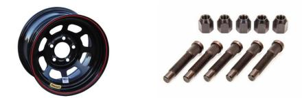
11.11 <u>An OEM aluminum wheel will be allowed for a minimum number of races to be</u> <u>determined by tech. After which the competitor must install the above racing</u> <u>wheel on the right side.</u>
