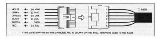
Above shows wiring order for connector installation on MSD 6AL and 6T Ignition Box
