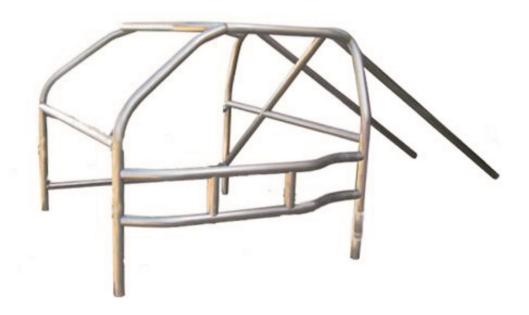
**N O T E**: Optional - Right side pipes may be in the form of an "X" or a single tube angled down from top of door on the right rear pipe to the bottom of the right front pipe.
