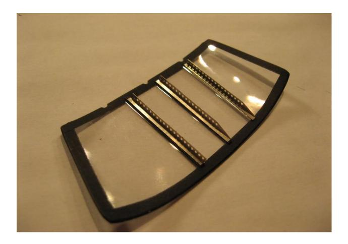
A Lexan windshield will be allowed. It must have a minimum of three steel evenly spaced braces installed in windshield opening to right of driver.
