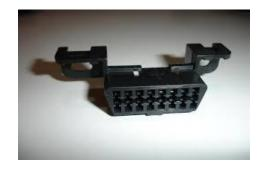
Vehicle OBD II diagnostic connector must be readily accessible and all terminals must be operating as OEM. A scan tool must be able to access the engine computer data.
